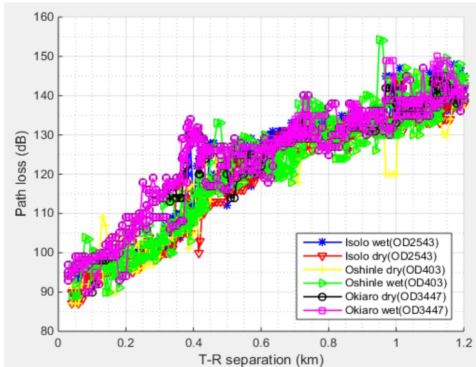
**Figure 2.** Seasonal variation of measured path loss values in different urban environments
