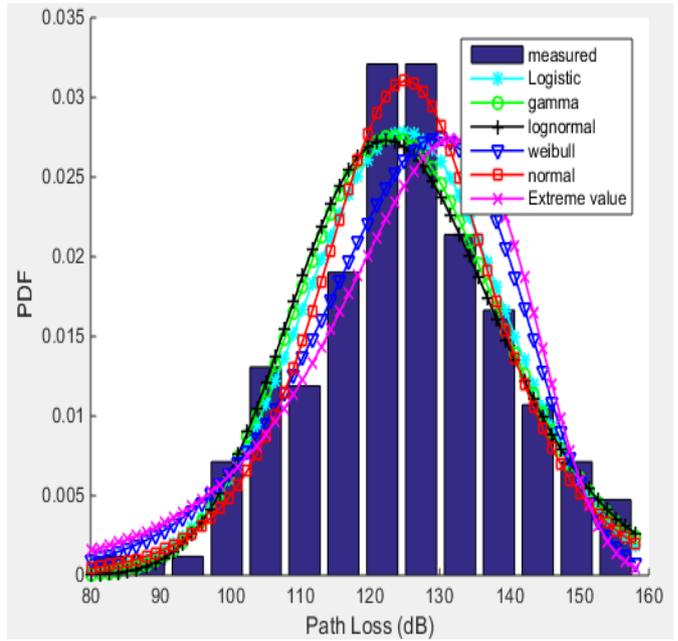
**Figure 6.** Fitting of probability distribution to the wet season measured path loss values in Akure urban environment.
