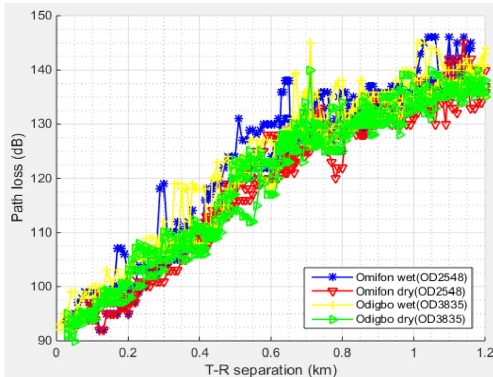
**Figure 4.** Seasonal variation of measured path loss values in different urban environments
