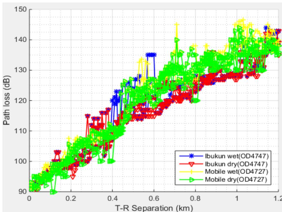
**Figure 3.** Seasonal variation of measured path loss values in different suburban environments
