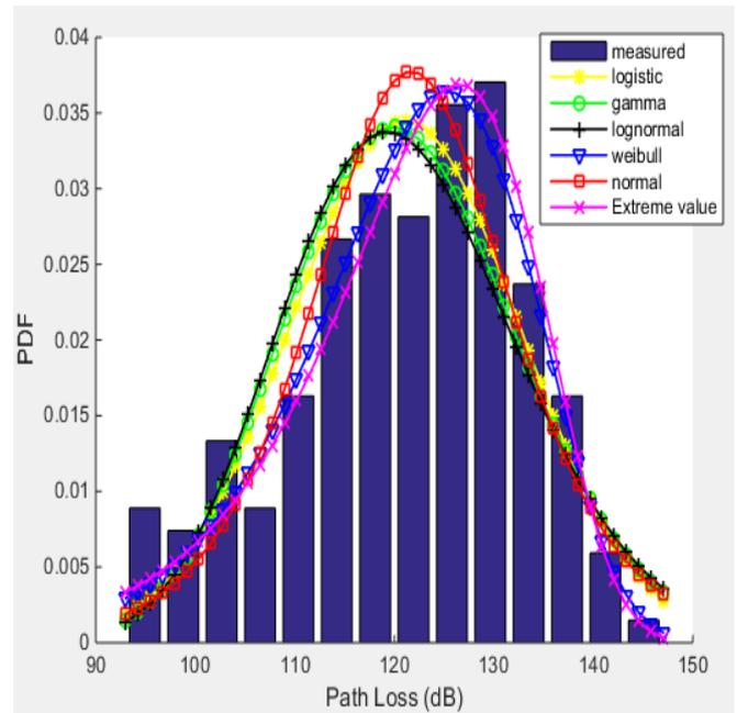
**Figure 10.** Fitting of probability distribution to the wet season measured path loss values in Omifon and Odigbo rural environments.
