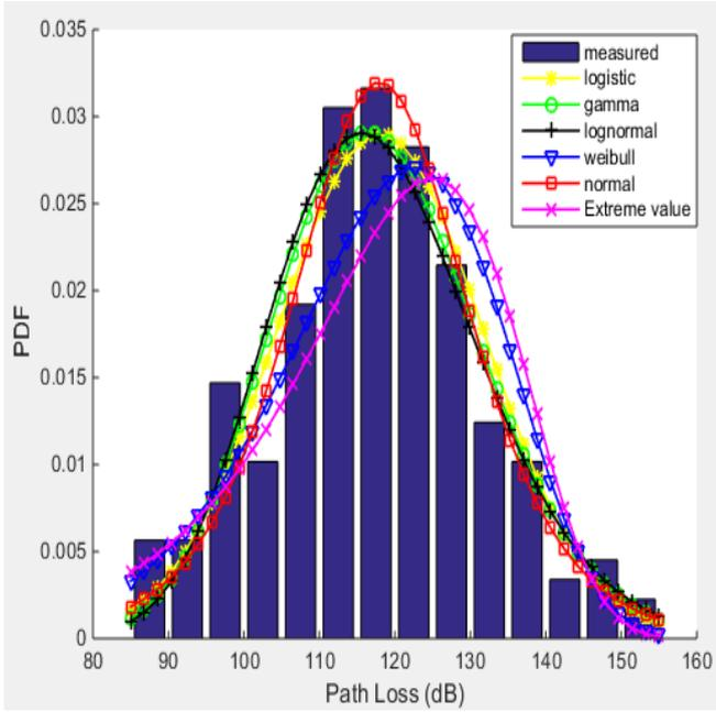
**Figure 5.** Fitting of probability distribution to the dry season measured path loss values in Akure urban environment.
