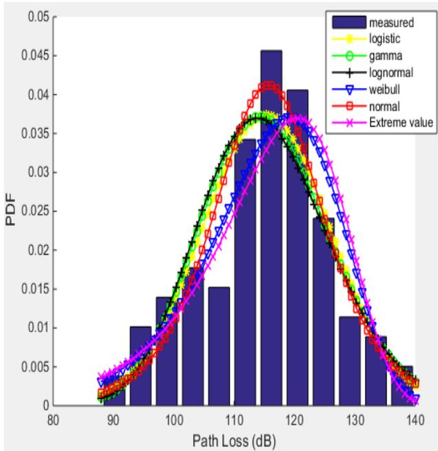
**Figure 9.** Fitting of probability distribution to the dry season measured path loss values in Omifon and Odigbo rural environments.
