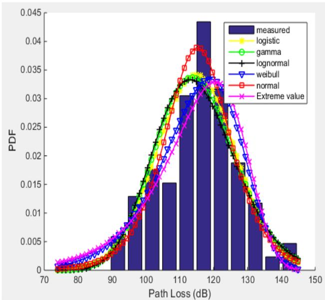
**Figure 7.** Fitting of probability distribution To the dry season measured path loss values in Ore suburban environments.
