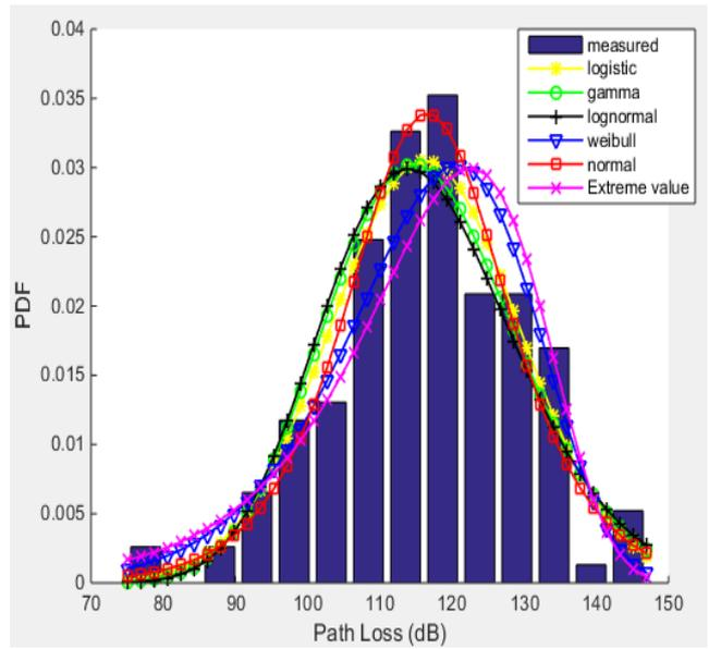
**Figure 8.** Fitting of probability distribution to the wet season measured path loss values in Ore suburban environment.
