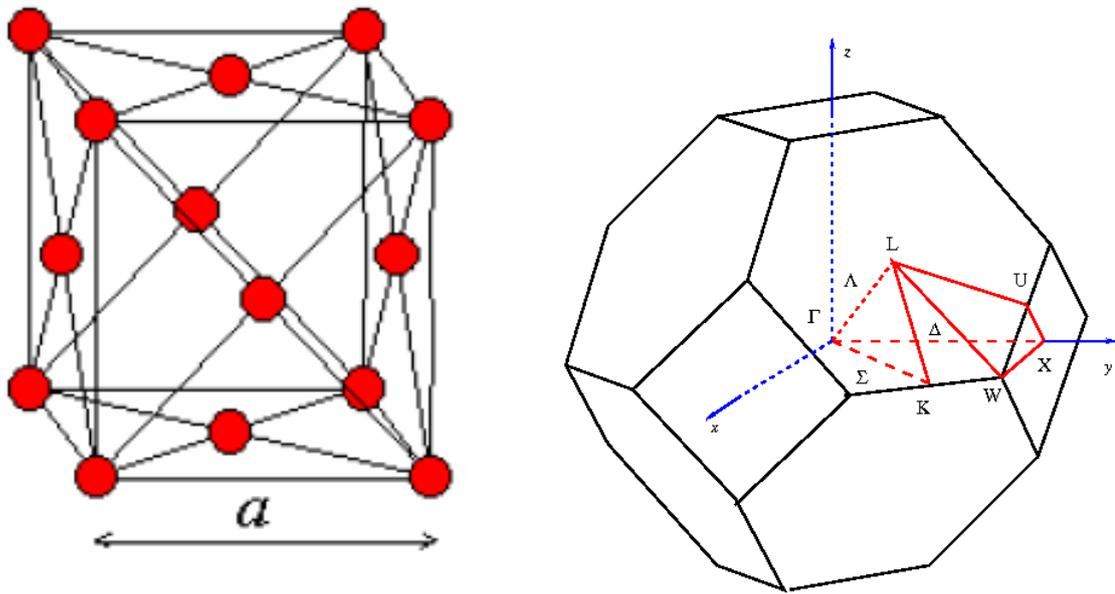
**Figure 2.** FCC lattice (left) and the first Brillouin zone (right).
