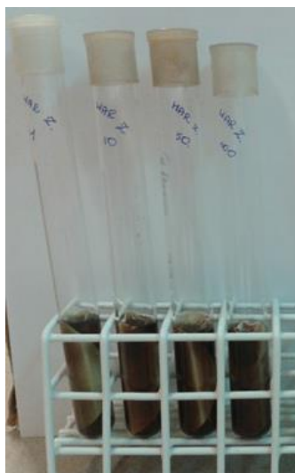
Figure 1. Semi-Fraser medium after incubation with visible filter discs. Listeria spp. hydrolyse the esculin from the semi-Fraser medium to esculetin and glucose. Esculetin reacts with the iron ions contained in the substratum, which results in darkening of medium.
