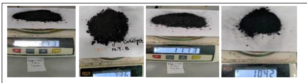
Figure 5. Pyrolysis of lignin (walnut shell, almond shell, neem tree bark, babool tree bark for catalyst preparation
