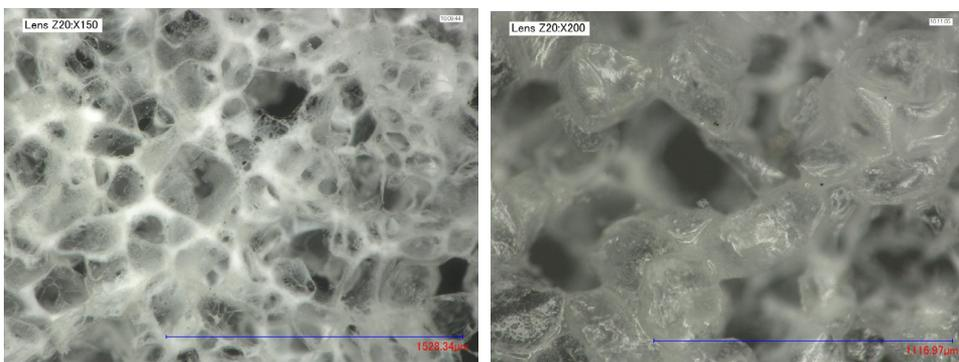
**Figure 7.** Scanning electron micrographs of the porous structures obtained by the porphor agent salt-leaching method.
