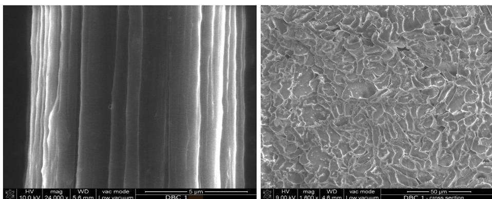
**Figure 3.** Micrographs of dibutylchitin fibres.
