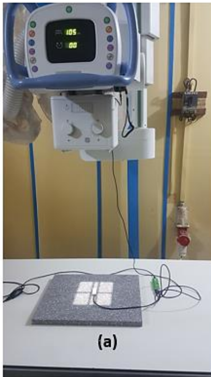
Figure 1. (a) Set-up for tube output, kVp, mAs, HVL measurements; (b) MagicMax display software from a PC.
