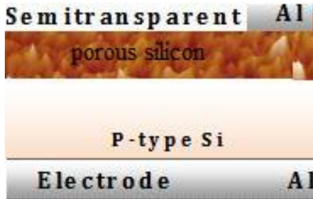
Figure 2. Cross-sectional view of Al/PS/p-Si/Al metal semiconductor metal structure
