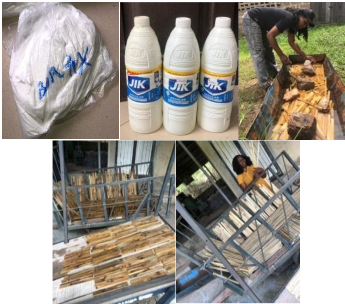
Figure 3. Treatment of Uniform Bamboo Strips Using Boric-acid and Jik (Sodium Hypochlorite) and Air-drying of Treated Bamboo Strips
