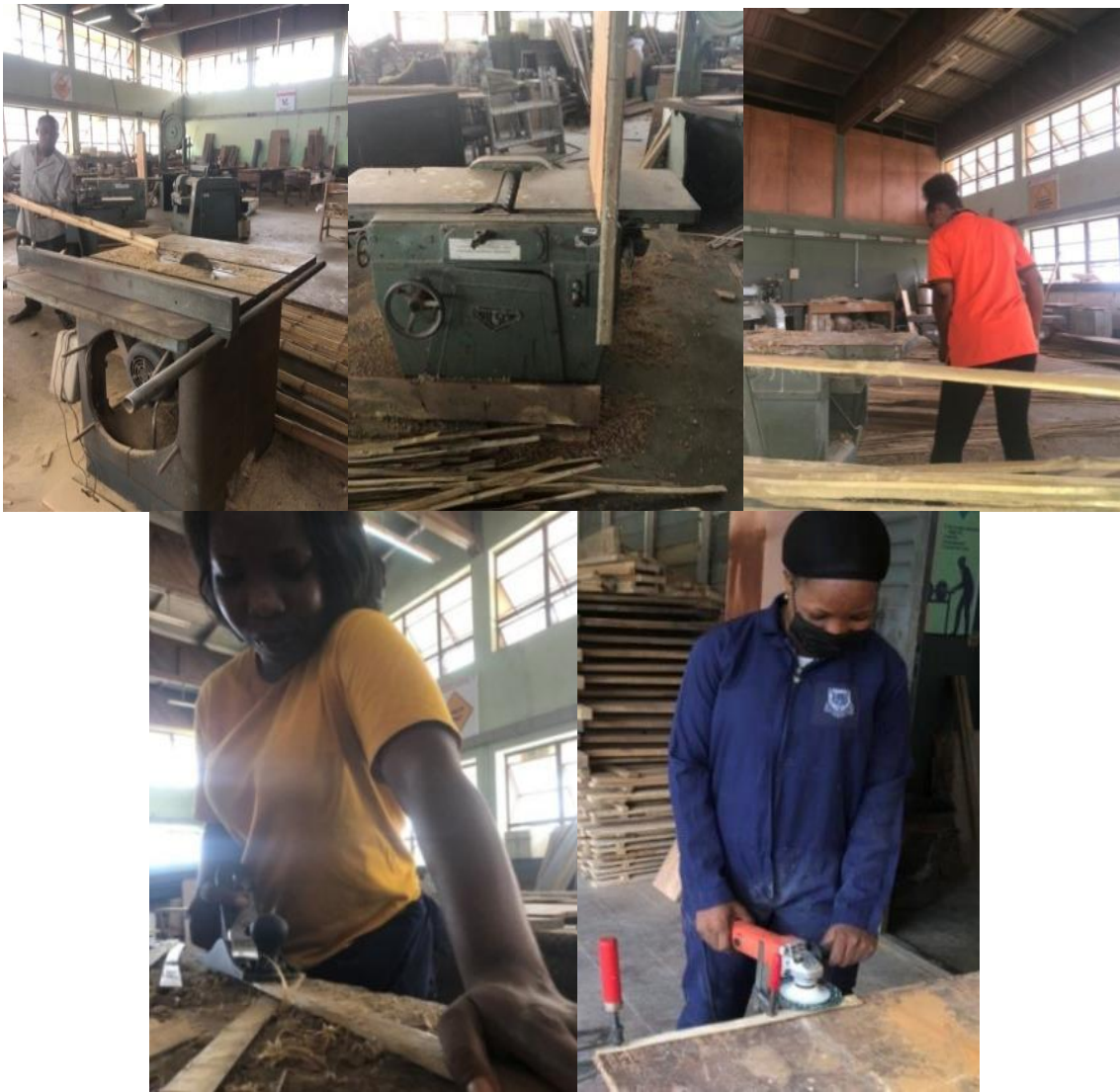
Figure 2. Planning of Bamboo Strips using Combined Thicknessing and Surface Planning Machine, Smooth Plain and Grinding Machine
