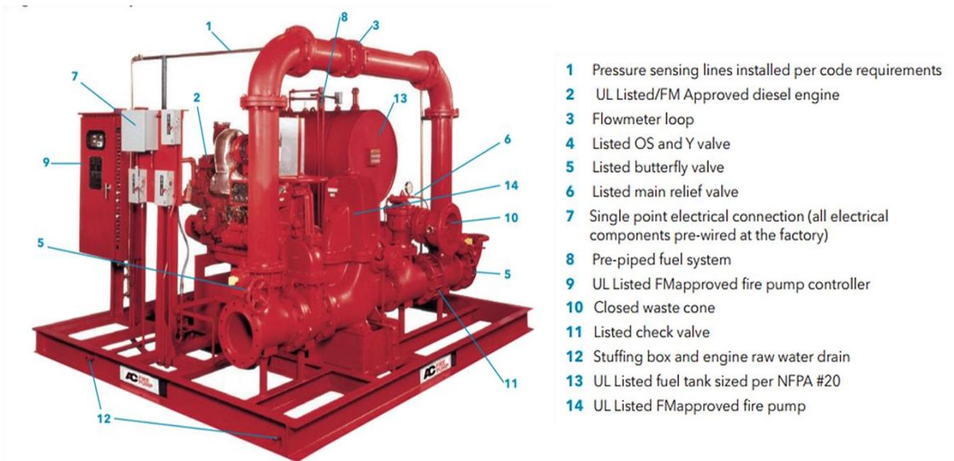
Figure 2. Fire pump (Fire Hydrant System) [WIKIPEDIA].
