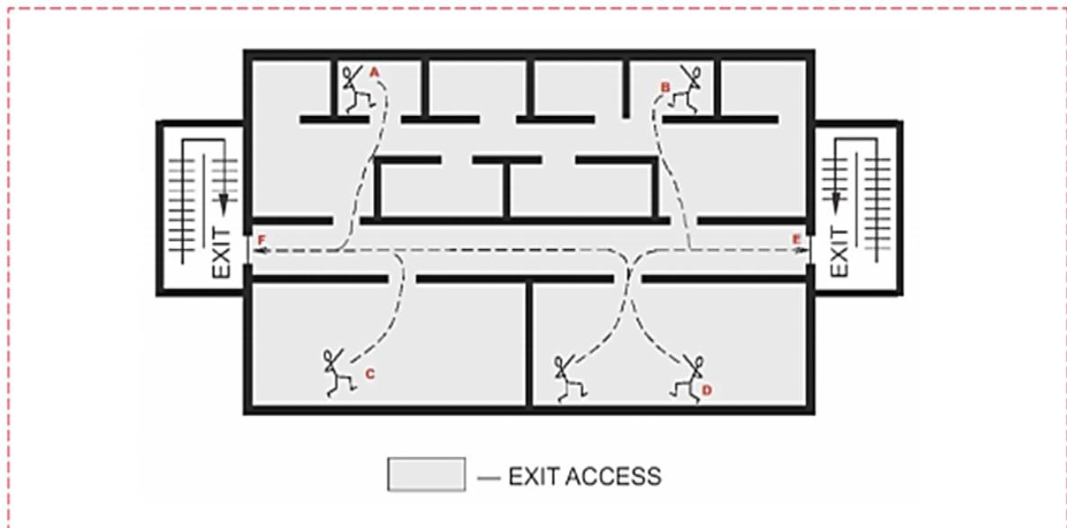
**Figure 5.** The short safe travel distance for fire safety [20].
