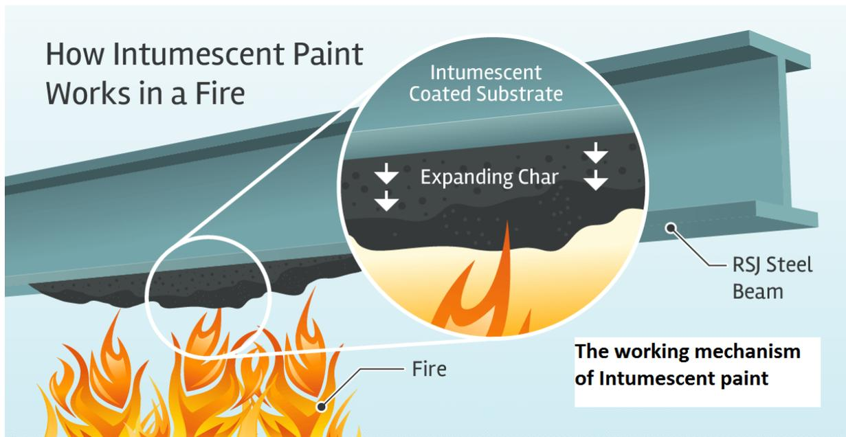
**Figure 7.** The working mechanism of intumescent paint [25].
