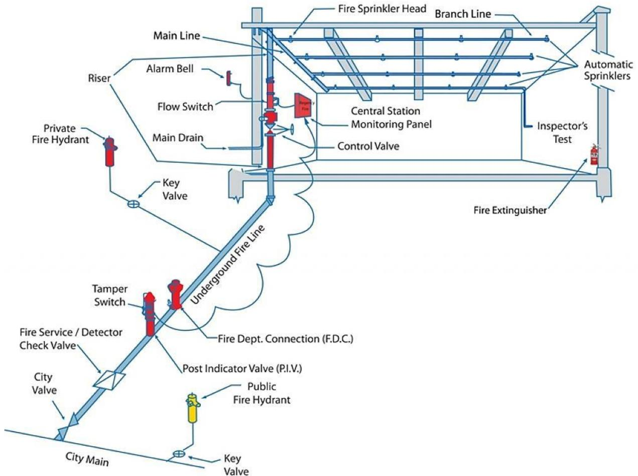
**Figure 4.** The pictorial view of the Automatic Sprinkler System [WIKIPEDIA].
