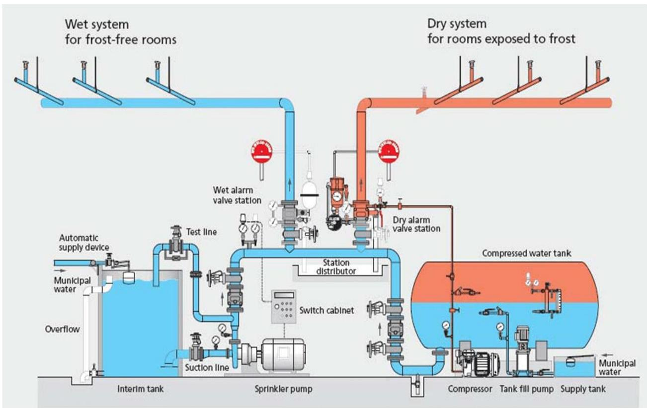
**Figure 3.** Dry & wet riser system [14].
