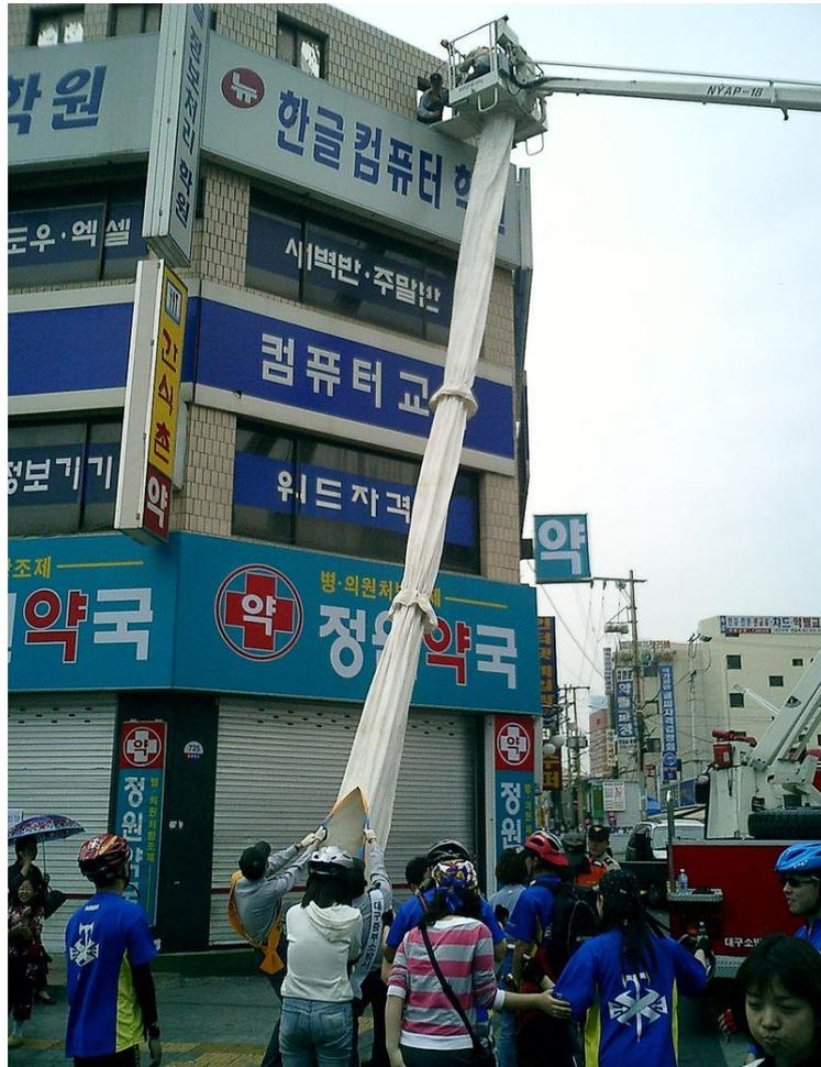
Figure 6. The escape chute system in Seoul, South Korea.
