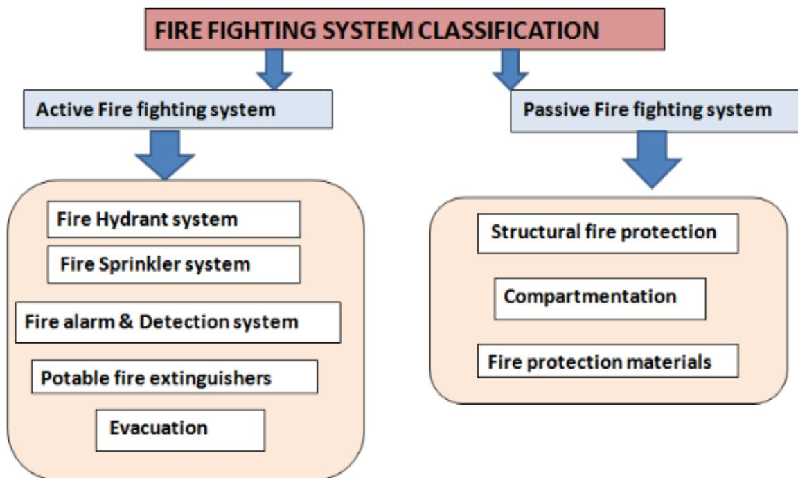
Figure 1. The firefighting system classification [6].
