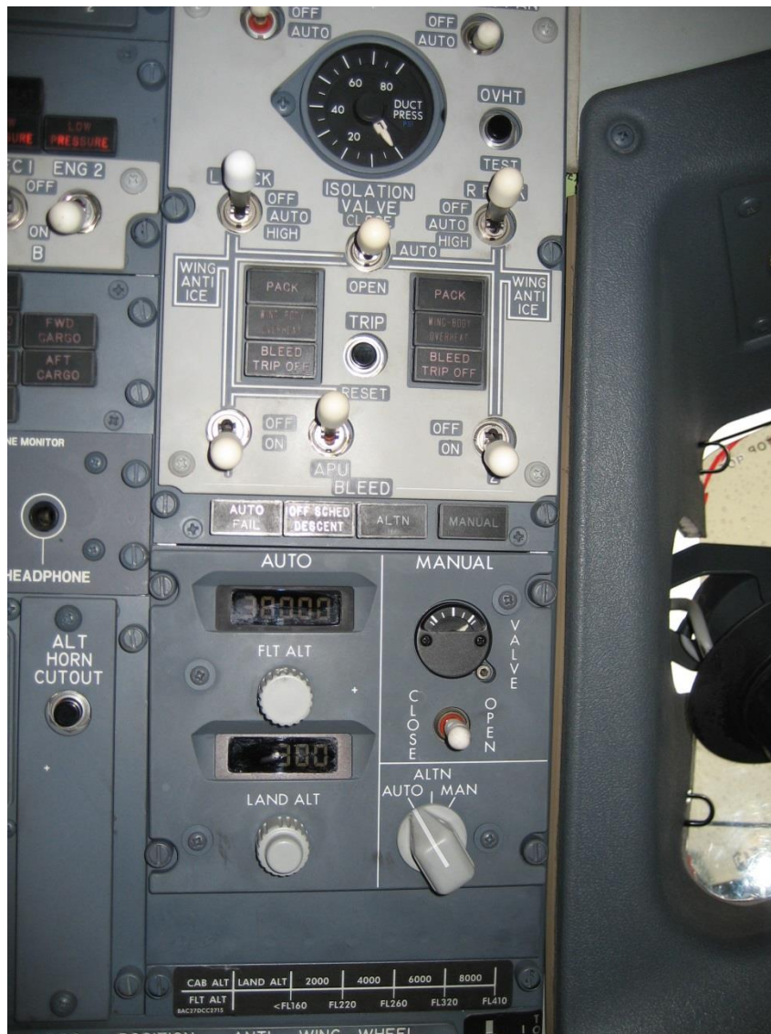
Figure 2. Environmental control system panel in a Boeing 737-800. By Wsombeck, released into the Public Domain, Wikimedia Commons.
