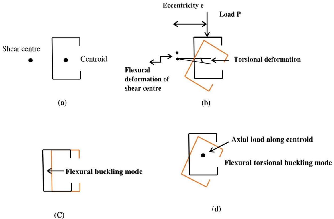
Figure 3. Typical torsional rigidity.
