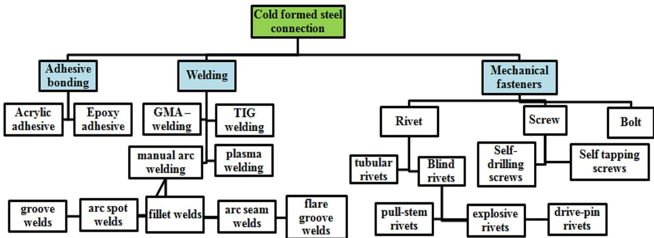
Figure 4. Cold formed steel connection
