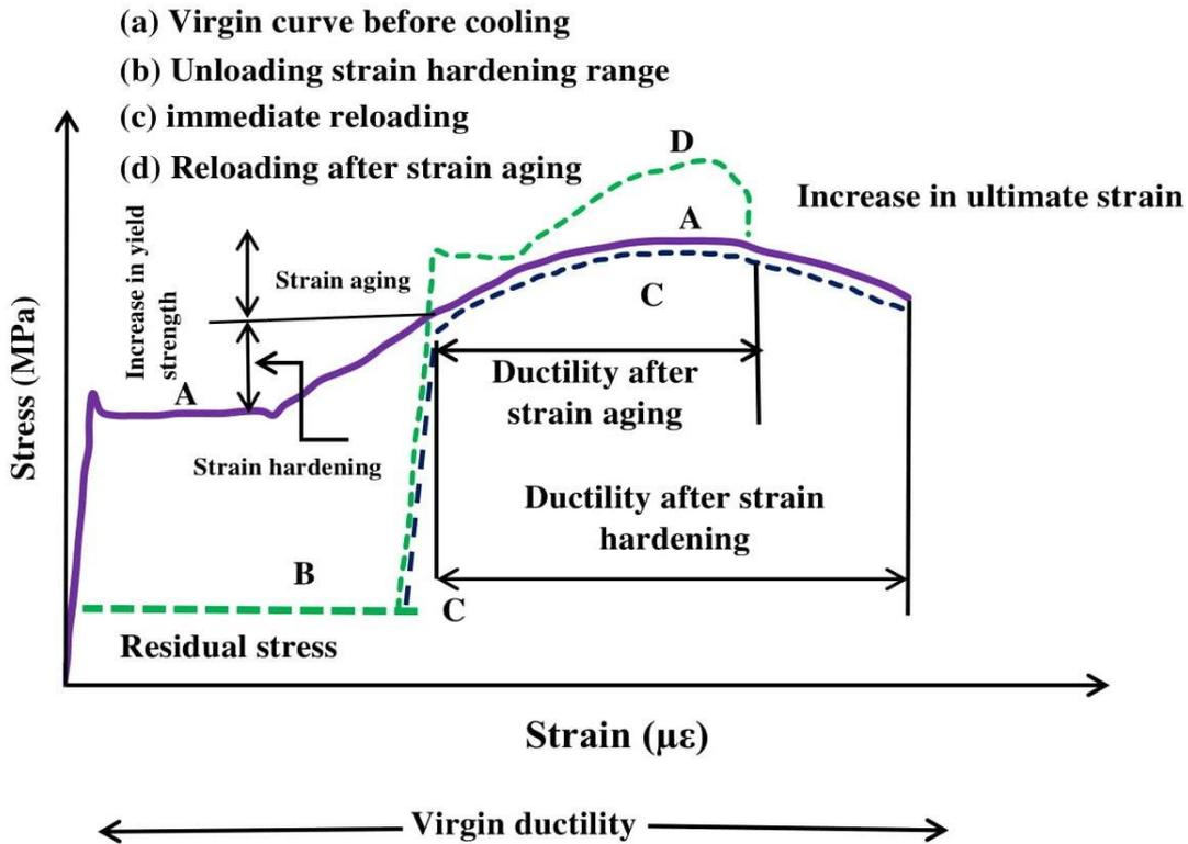
**Figure 1.** Effects of strain hardening and strain aging on typical stress-strain characteristics of structural steels.
