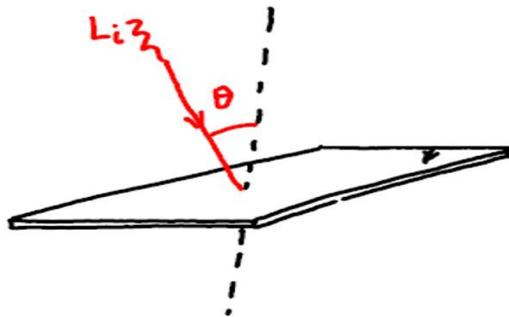
**Figure 6.** Incident insolation at an angle at solar panel due to its tilt
