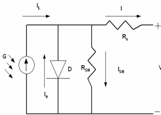
**Figure 4.** Circuit diagram of PV module
