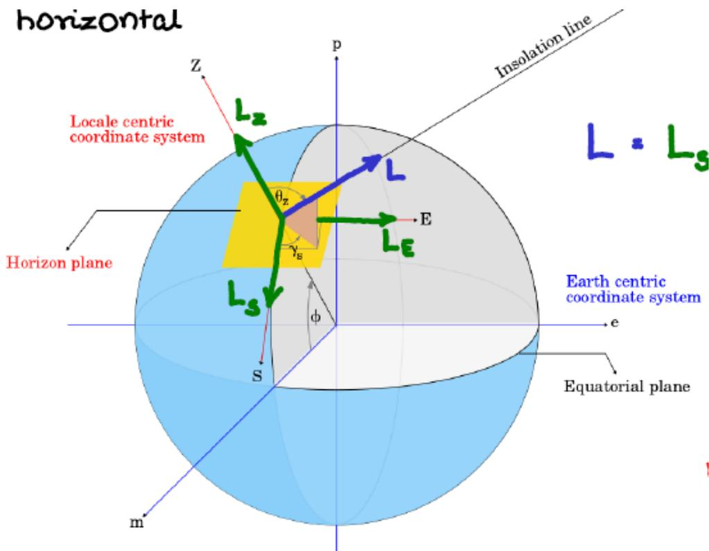
Figure 1. Insolation on a horizontal flat plate
