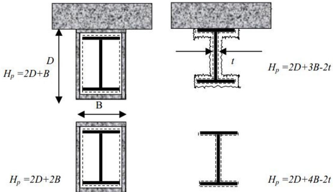
Figure 3. Typical values of HP of fire protected steel sections [9].
