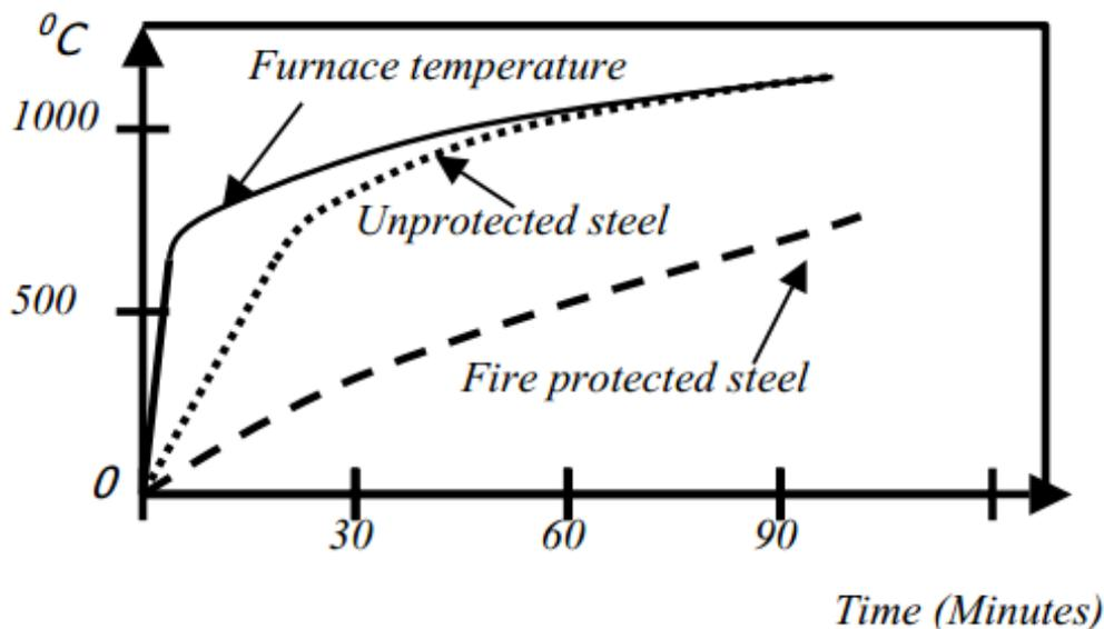
Figure 1. Rate of heating of structural steel work [4].
