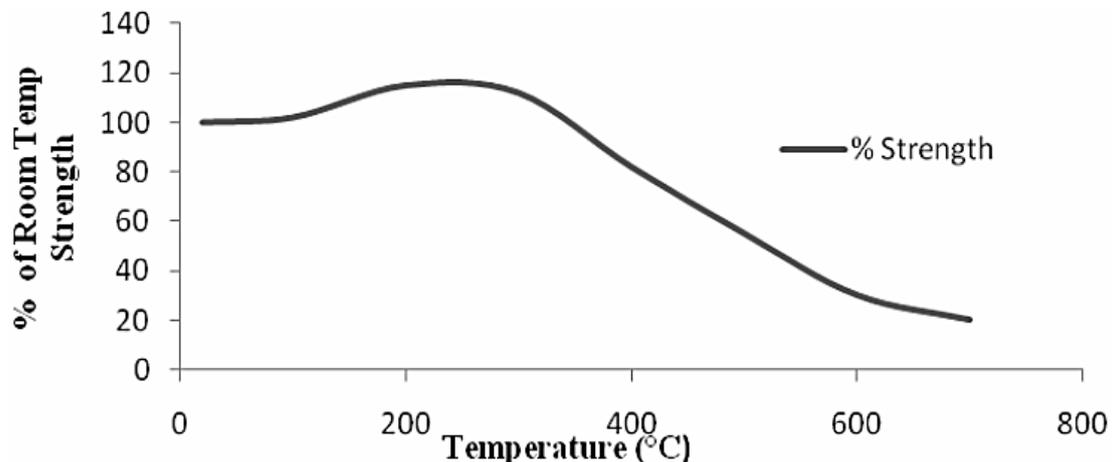
**Figure 2.** The relative strength of mild steel as a function of temperature to that of mild steel at room temperature [5].
