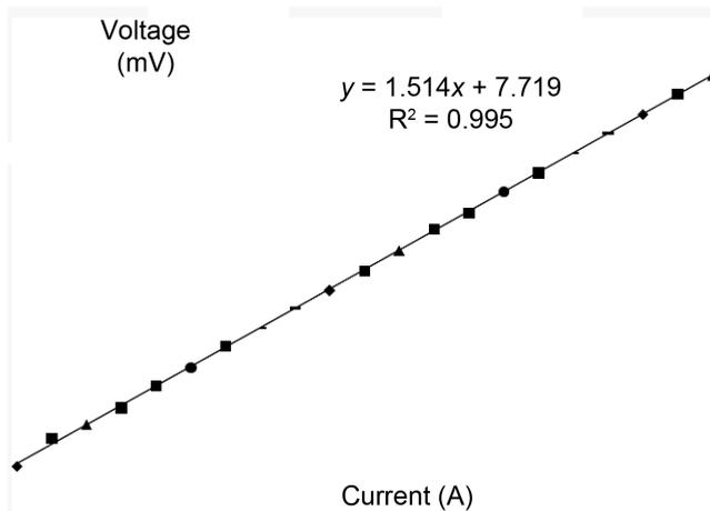
Fig. 6. Experimentally measured characteristic of the developed DC current transformer with its linear fit
