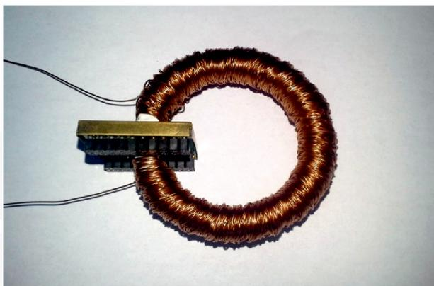
Fig. 4. Constructed DC current transformer
