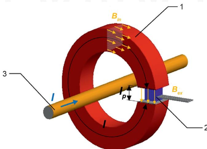
Fig. 1. Schematic diagram of current sensor: 1 – magnetic field concentrator, 2 – Hall sensor, 3 – wire under test
