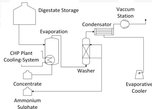
Fig. 7. Working principle of a single-step vacuum evaporation system
