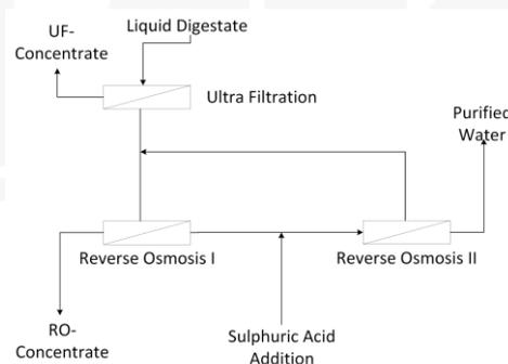
Fig. 8. Membrane process for total digestate treatment
