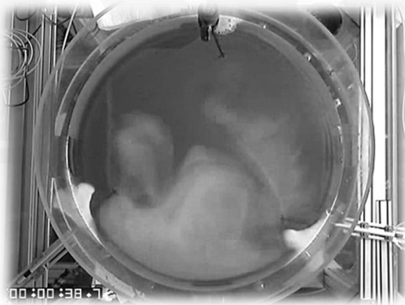
Fig. 13. Flow field at a xanthan gum of 3 g/kg (stirrer speed: 3000 rpm; azimuth angle: 65°)
