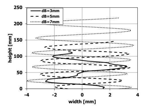
Fig. 1. Rising paths of three differently sized bubbles for a rising duration of 1 second each in a channel with a depth of  $d_c = 3 \text{ mm}$  (from OpenFOAM simulation)
