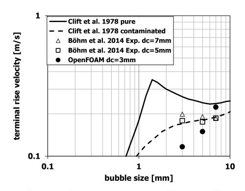
Fig. 4. Terminal rise velocity for free rising bubbles in pure and contaminated water (experimental data, [1]), in a confining rectangular geometry with channel depths of  $d_c = 5 \text{ mm}$  and 7 mm (experimental data, [5]) and for a channel depth of  $d_c = 3 \text{ mm}$  (OpenFOAM)
