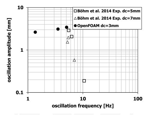
Fig. 2. Oscillation amplitude over oscillation frequency in a confining rectangular geometry with channel depths of  $d_c = 5 \text{ mm}$  and 7 mm (experimental data, [5]) and for a channel depth of  $d_c = 3 \text{ mm}$  (OpenFOAM)
