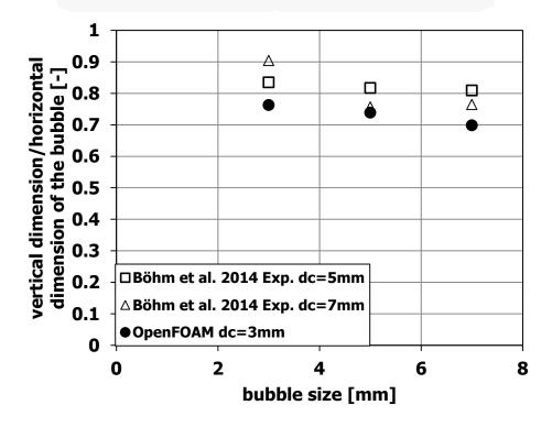
Fig. 3. Ratio of the horizontal and vertical dimension of the bubble over the bubble size in a confining rectangular geometry with channel depths of  $d_c = 5$  mm and 7 mm (experimental data, [5]) and for a channel depth of  $d_c = 3$  mm (OpenFOAM)
