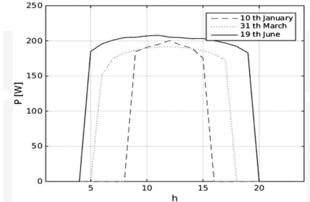
Fig. 1. The hourly average value of power generated by PV module with angle of elevation 30° and south orientation
