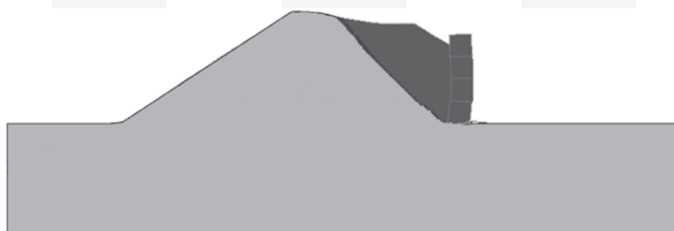
Fig. 4. Sliding surface for embankment with 4 gabions
