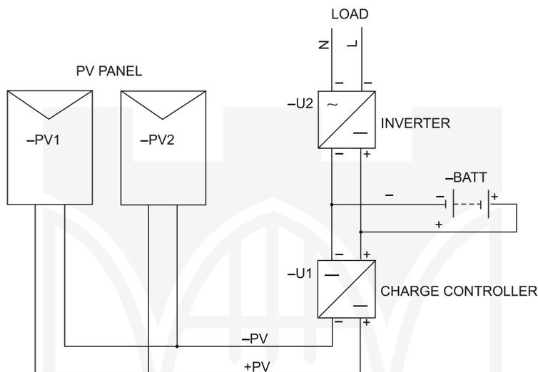
Fig. 3. Electrical diagram of the PV power supply for laboratory installation
