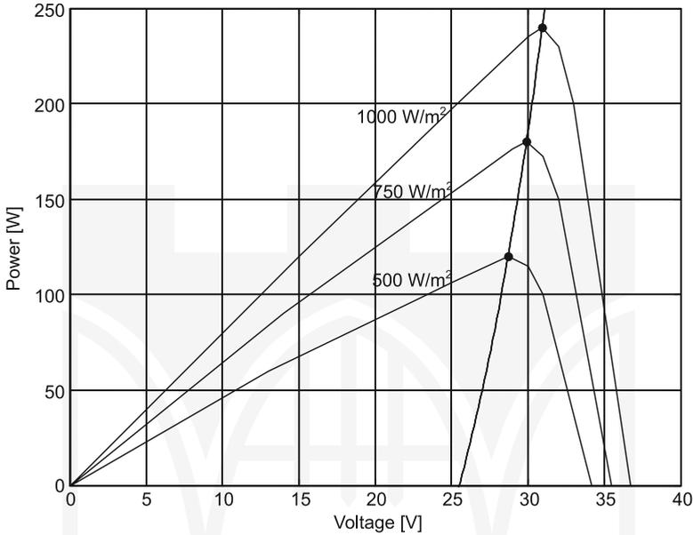
Fig. 2. An example of a voltage – power characteristic of PV panels for different values of irradiance (the dashed line represents MPP)
