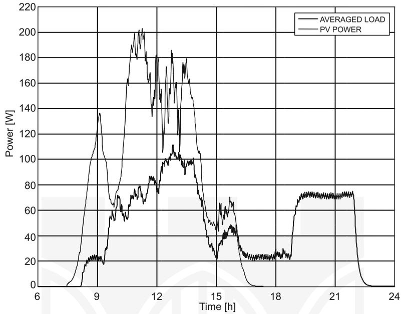
Fig. 6. Example of comparison of the power generated by the PV cells and consumed by the HVAC system
