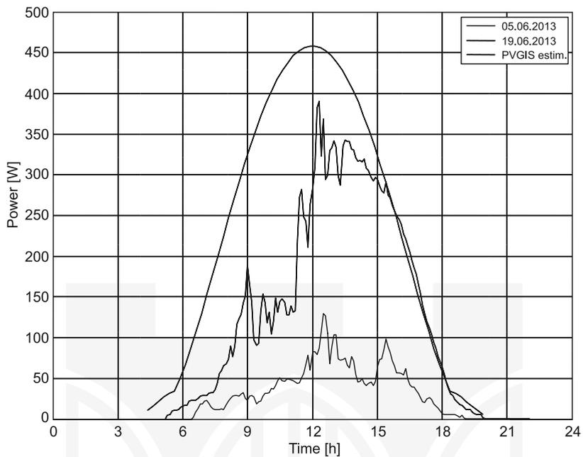
Fig. 4. Comparison of generated power for sample sunny and cloudy days (summer)
