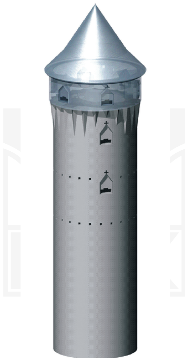
III. 3. Lipowiec Castle, 3D model of the tower from the level of the courtyard. Reconstruction of the upper floor over the corbels has been performed according to the drawings by Janusz Bogdanowski (museum of the Lipowiec Castle), drawn by J. Czechowicz
