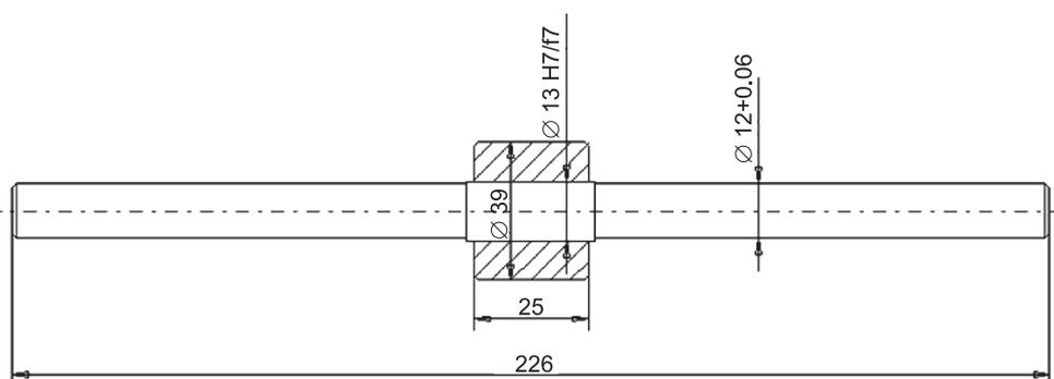
Fig. 2. Dimensions of the sample for modelling tests
