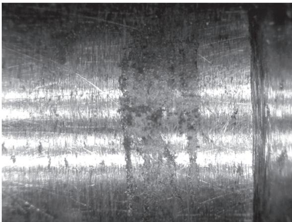
Fig. 5. Macroscopic picture of fretting damage on shaft surface – corrosion marks characteristic of fretting, magn. ca. 15×
