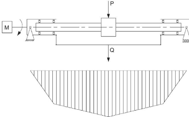
Fig. 3. Specimen loading and bending moment distribution
