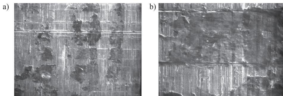
Fig. 8. Scanning picture of fretting wear on shaft seat surface, press-fitted joint, a) magn. 200 $\times$  – wear areas scattered on the surface in the form of oxidised ridges, b) magn. 1000 $\times$  – material ridges, plastic deformations, pits
