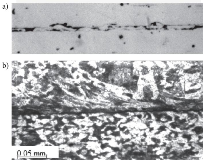
Fig. 9. Shaft-sleeve interface, press-fitted joint, magn. 320 $\times$ , a) non-etched, b) etched
