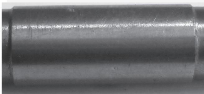
Fig. 11. Surface of steel shaft lubricated with Glacier grease after fatigue tests – no fretting wear, magn. ca. 3×
