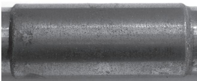
Fig. 10. Surface of molybdenum shaft after fatigue tests – no fretting wear, magn. ca. 3×
