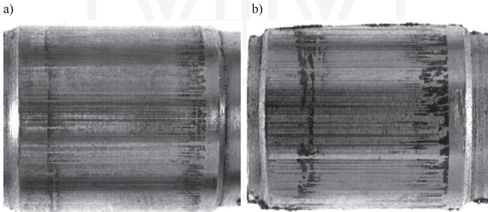
Fig. 7. Photographs of shaft seat after wear tests, press-fitted joint, magn. 4×, press-fitting: a) – 0,02 mm, b) – 0,04 mm.
