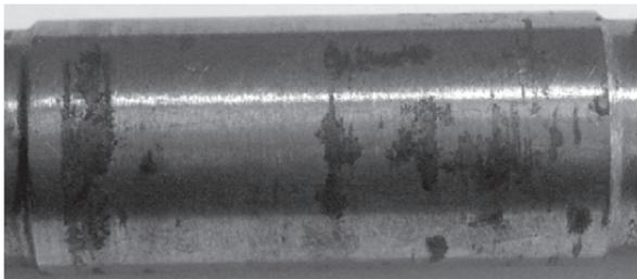
Fig. 4. Shaft surface after fatigue testing – clear marks of fretting wear on shaft edges, with decrease intensity inwards, magnified ca.  $3\times$
