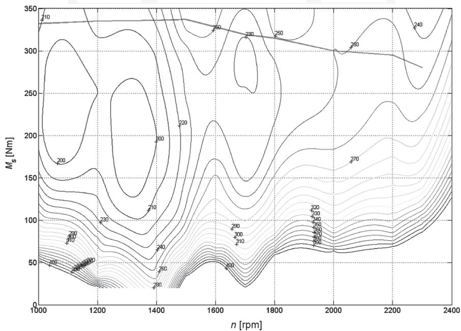
Fig. 2. Versatile characteristics of engine with flameproof inlet-outlet system [2]
