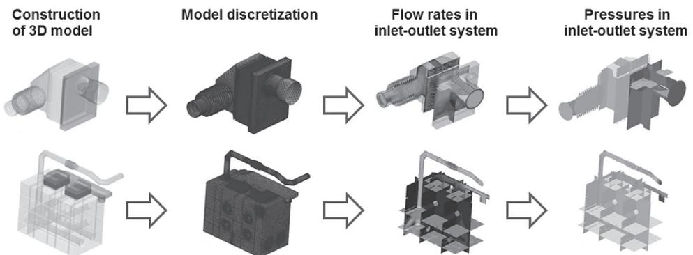
Fig. 4. Simulation tests of inlet-outlet system with use of CFD software programme [3]
