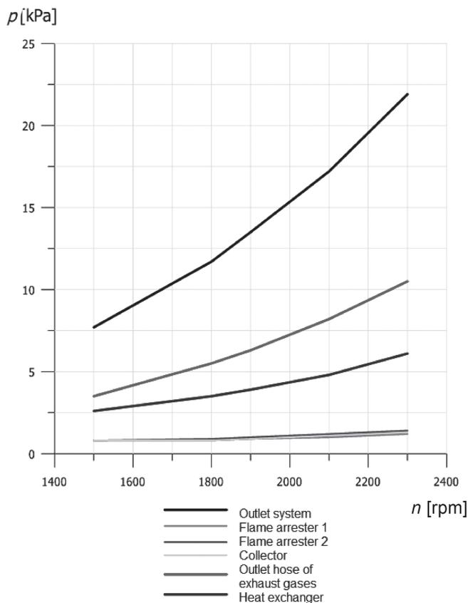
Fig. 5. Flow resistance in each component of the outlet system [3]
