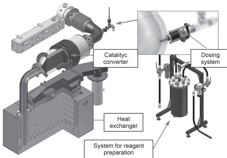
Fig. 7. Systems for processing the exhaust gases in the outlet system [5]
