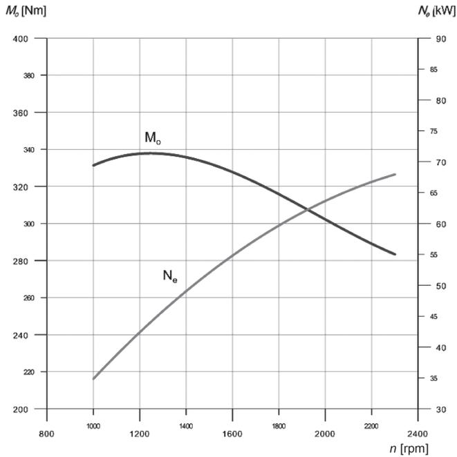
Fig. 3. External characteristics of diesel engine [4]
