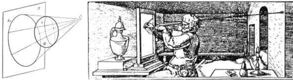
III. 1. On the left – significant outline on a sphere and ostensible outline on the projection plane, on the right – the technology of outlining objects on the example of rotational solid [6]
