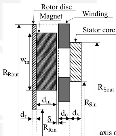
Fig. 2. Single-stator, single-rotor topology of single-phase axial-flux magnet generator
