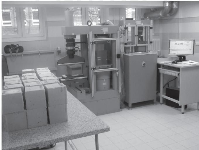
III. 3. Measurement of compressive strength
