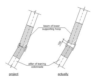
III. 9. Knot of pressing the pillars of leaning colonnade with iron concrete beams of lower supporting hoop of cover of cooling tower station #1 Kyiv Combined heat and Power Plant 6
