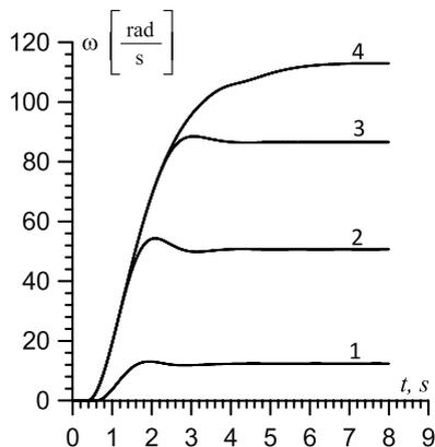
Fig. 3. Time dependence of the speed's rotation of the motor for different values of the input voltage  $u_1$ : 1–5 V, 2–10 V, 3–15 V, 4–20 V
