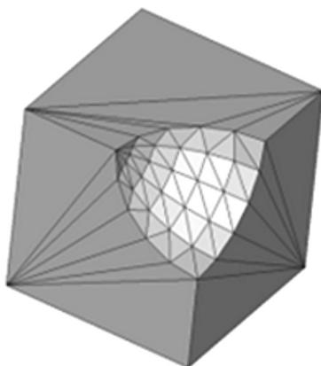
Fig. 4. 3D model surface saved in STL format [2]
