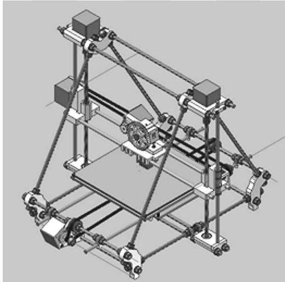
Fig. 6. The assembly of the 3D RepRap printer
