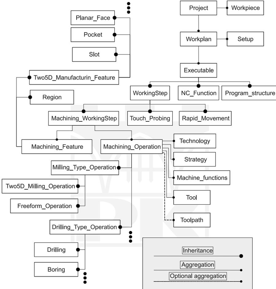
Fig. 2. The simplified view of STEP-NC data structure
