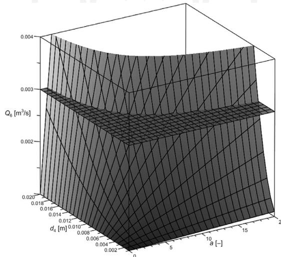
Fig. 4. The volumetric flow rate at the outlet  $Q_6$  [m<sup>3</sup>/s] dependence of nozzle's number  $a$  [-] and nozzle's diameter  $d_4$  [m]
