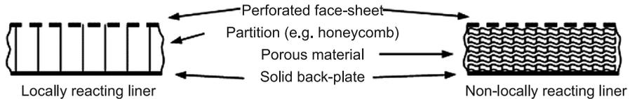
Fig. 9. Two types of acoustic liners as described in [3]
