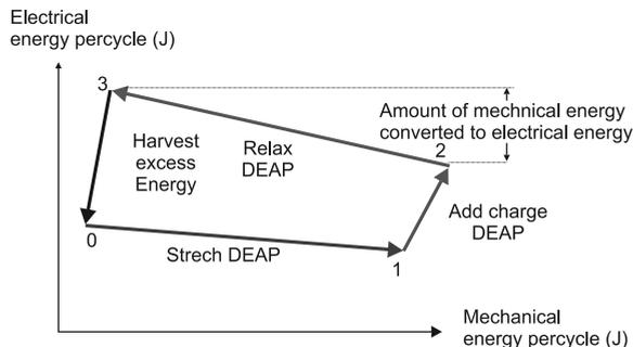
Fig. 2. Energy harvesting cycle of a dielectric elastomer [9], DEAP – dielectric electroactive polymer
