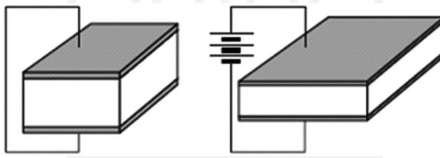
Fig. 1. Mechanical deformation of a dielectric elastomer under DC actuation voltage
