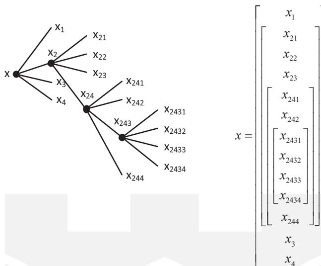
Fig. 1. Example of a Fuzzy Signature Structure
