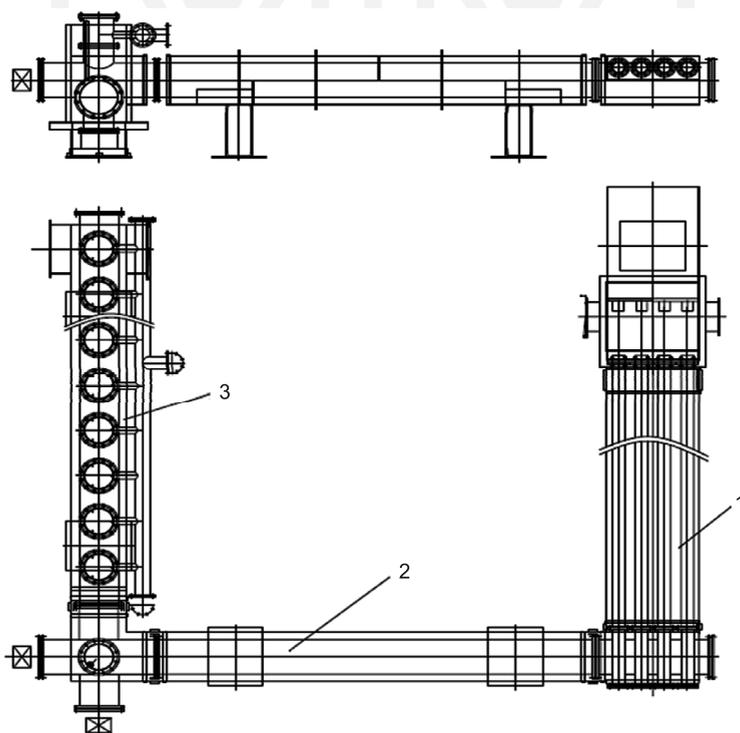
Fig. 3. Depolymerization block (1 – heater, 2 – melter, 3 – cracking furnace)
