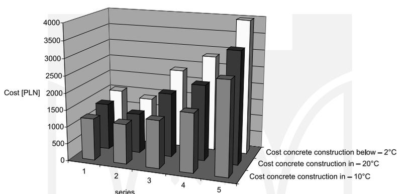
Fig. 1 Cost calculation results for producing 1 m<sup>3</sup> of concrete construction in -10°C, -20°C and below -20°C (series: 1 – Concrete admixtures, 2 – Hot concrete mix, 3 – Hot mix and thermal insulation, 4 – Hot mix and heated shelter, 5 – Hot mix and heating mats)
