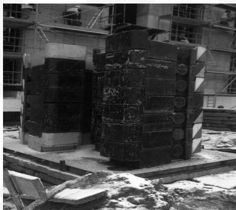
Fig. 2. A test load of the slope with ballast
