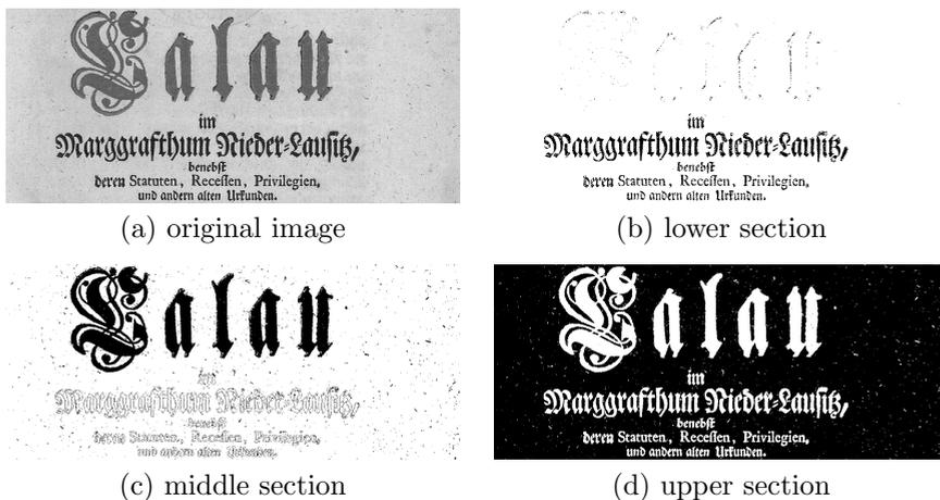
Figure 2. Multilevel binarization of the P03 image.
