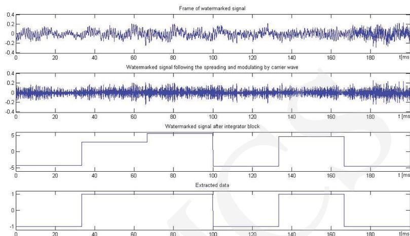
Fig. 8. Signal curves in the watermark extractor.
