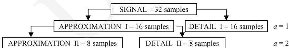
Procedure scheme is simple. Let us assume, that input signal consists of 8 samples  $I_0, \dots, I_7$ . Having wavelet coefficients  $H_0, H_1, H_2, H_3$  and scaling coefficients  $G_0, G_1, G_2, G_3$ , we have to multiply the signal through appropriate matrix:
