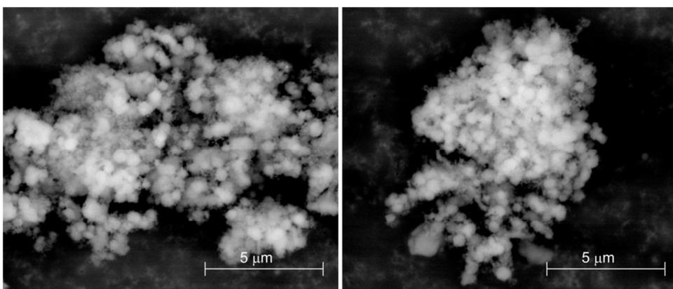
Fig. 6. Representative SEM images of MCM-41 silica material.
