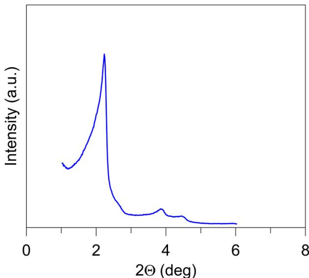
Fig. 5. X-ray diffraction pattern of MCM-41 silica under study.
