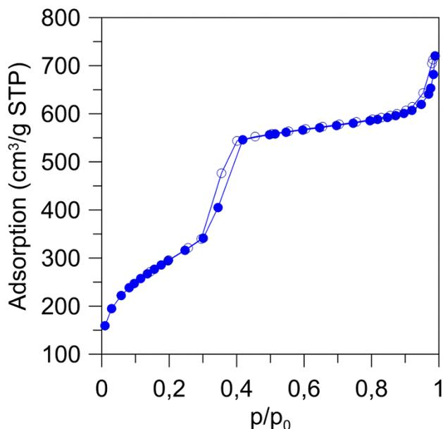
Fig. 3. Nitrogen adsorption (full points)/desorption (open points) isotherms at  $-196^{\circ}\text{C}$  of MCM-41 silica.
