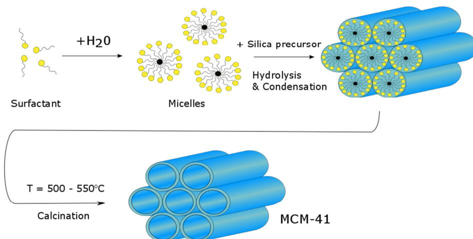
Fig. 1. Scheme of synthesis the MCM-41 silica material.
