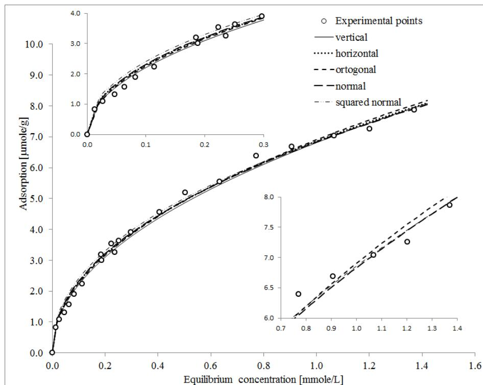
Fig. 3. Plots of optimized Freundlich isotherms for different error functions (pH = 6.1).
