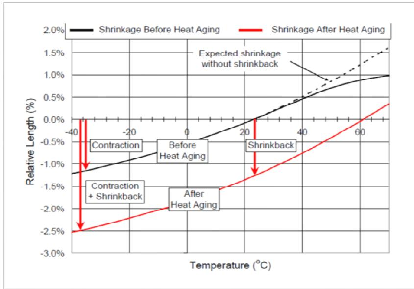
Fig. 2. Bill Hurley Corning – TMA measurement of PE cable jacket [13].
