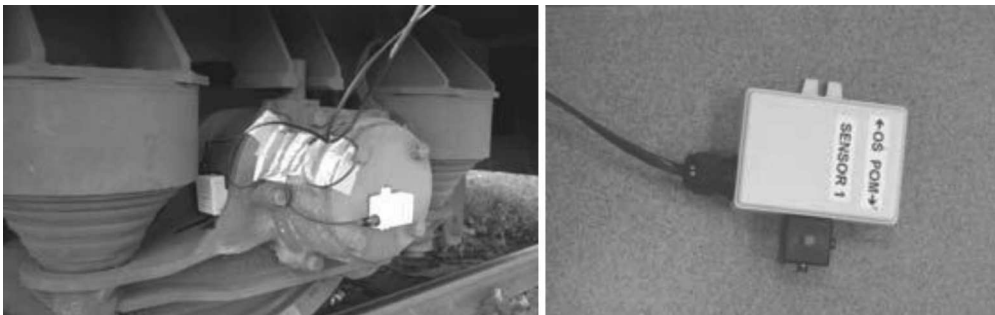
Fig. 5. Location of accelerometers on bearing box
