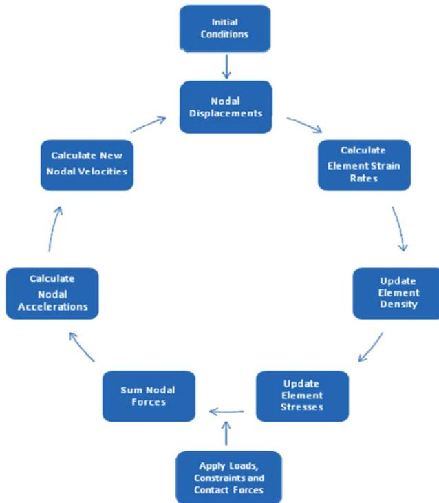
Fig. 2. Computation procedure scheme used in LS-DYNA computer program.
