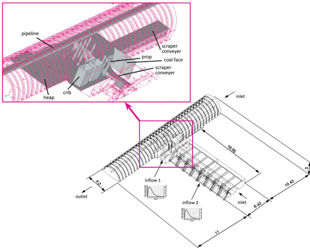
Fig. 1. The intersection of the CW-4 longwalls – a model
