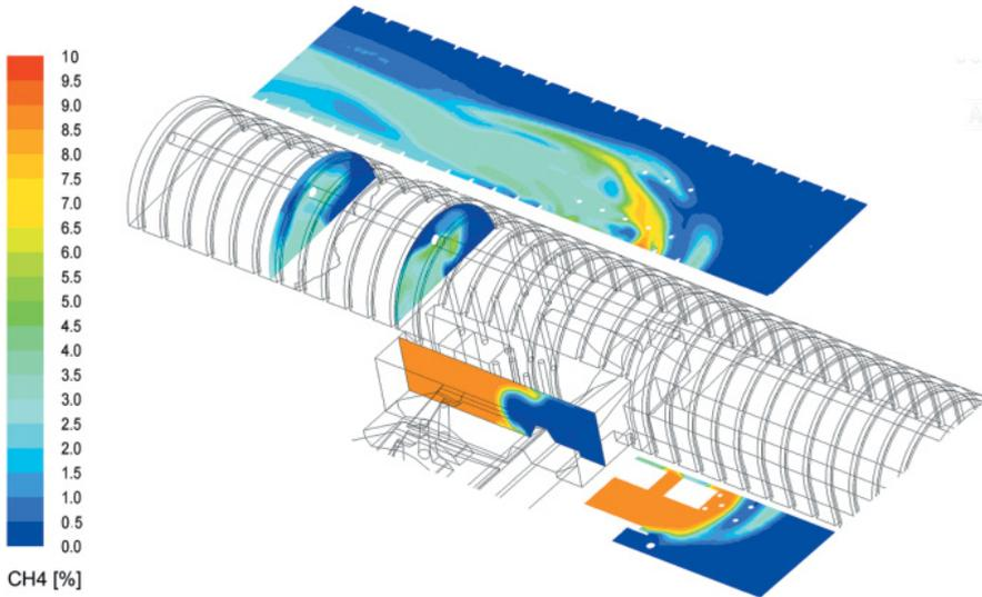
Fig. 5. The stationary field of methane concentrations for the steady maximum inflow of 27 m<sup>3</sup>/min – the *k-ε* model
