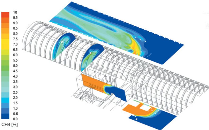
Fig. 6. The stationary field of methane concentrations for the steady maximum inflow of 27 m<sup>3</sup>/min – the *k-ω* SST model
