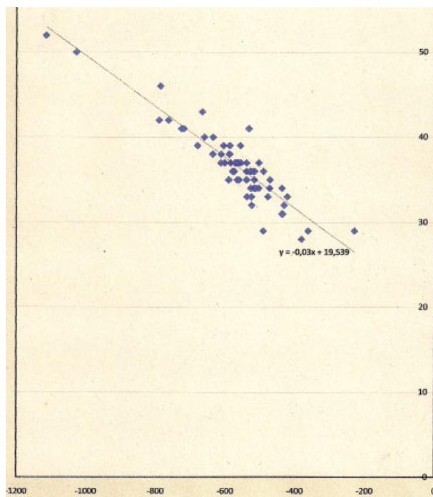
Fig. 3. Dependence of temperature on depth from the measurements of maximum temperature in mine borings.
