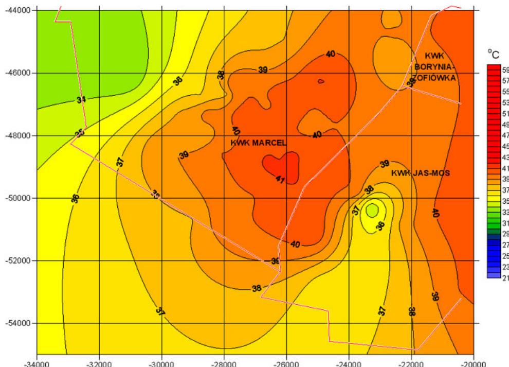
Fig. 8. Map of isothermal lines of the primary rock temperature at the level of -650 m in the border area
