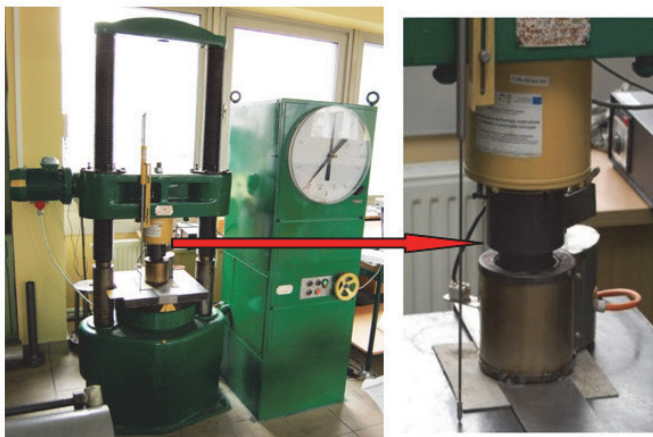
Fig. 2. The test station to perform the upset forging test – set of tools used in the process of upset forging at higher temperatures on a hydraulic press of maximum rated force 1MN
