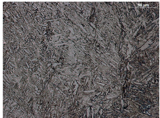
Fig. 5. Martensite (aprox. 70%) in weld after welding with micro-jet cooling (argon as micro-jet gas), magn. 500x
