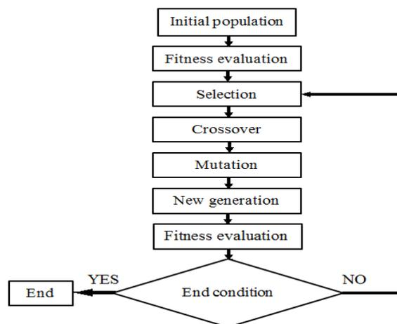
Fig. 7. Simplified graphical representation of the genetic algorithm.
