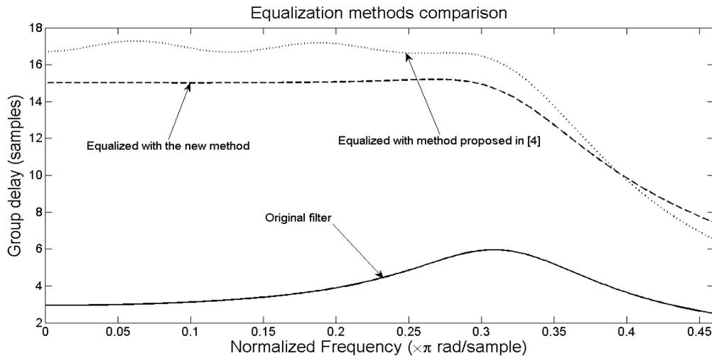
Fig. 6. Comparison of the presented method with the one proposed in [4] for the 5<sup>th</sup>-order Butterworth filter.
