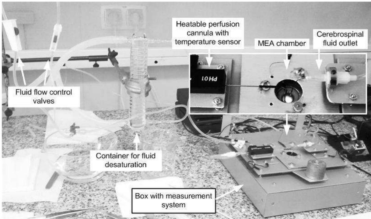
Fig. 14. Laboratory setup for multichannel *in vitro* multichannel neural activity recording using an MEA.
