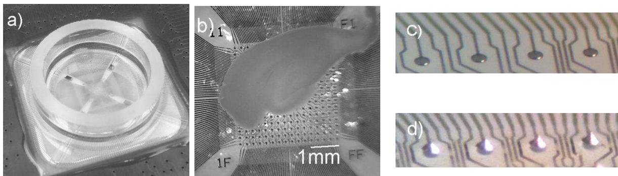
Fig. 5. Multi-electrode array for *in vitro* experiments realised on glass substrate. a) MEA mounted on PCB and surrounded by glass fringe creating a chamber for liquid. b) MEA with hippocampus tissue slice. c) planar electrodes. d) tip shaped electrodes. (Photos taken from the presented system).
