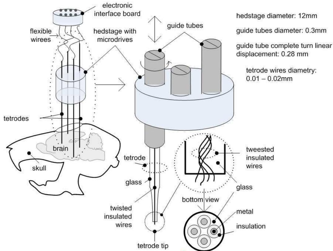
Fig. 2. Scheme of setup for *in vivo* multi-point neural activity recording by using tetrodes. Exemplary dimensions of key elements are taken from [10]. (The author's drawing).
