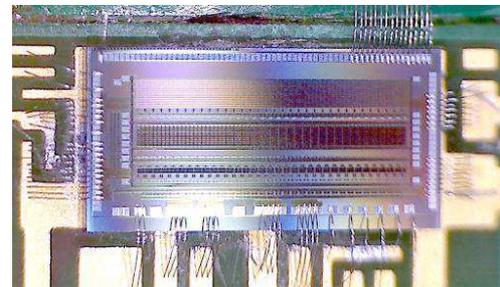
Fig. 8. Multichannel ASIC for neurobiological signal conditioning.
